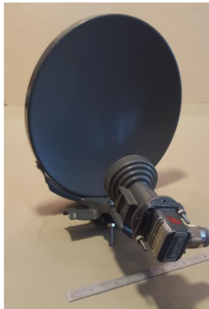
8" Offset Fed Dish G = 25 dBi 3dB Beamwidth \sim 9 deg
