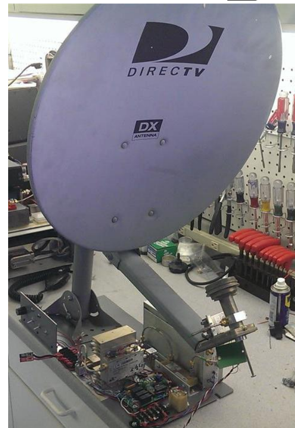
18" Offset Fed Dish G = 32 dBi 3dB Beamwidth \sim 4.3 deg
