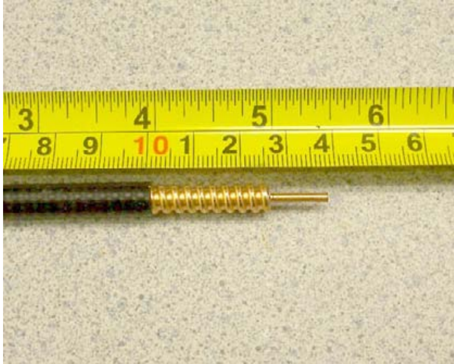
Prepared FSJ1-50 for an N-connector
