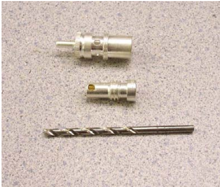
#28 drill hole in reducer
