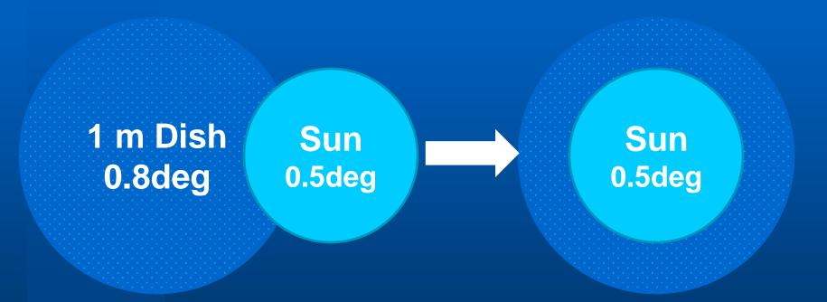
Increasing Antenna Gain WILL Increase Noise Until BW Equals Sun Diameter
