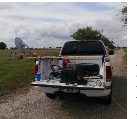
18 inch offset fed dish 400 mW Qualcom PA Double balanced mixer with no RF amplifier on receive
